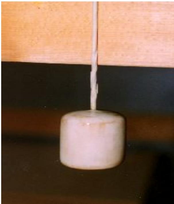
Float. Wire is 1/8" diameter stainless steel embedded in the eurothane foam core. Six 1/2" thick rectangles of foam were epoxied together then contoured by hand to create the float shape. One layer of a 4 oz. fiberglass cloth was applied over the foam followed by a couple applications of microballons in
