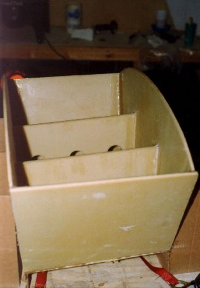
Tapes are wetted out and peel plied. I should mention here the importance of peel ply. It is used on all panel surfaces and tapes to insure the fibers are properly wetted out and laying flat which prevents fuel from wicking along the fibers and finding a path out of the tank.
