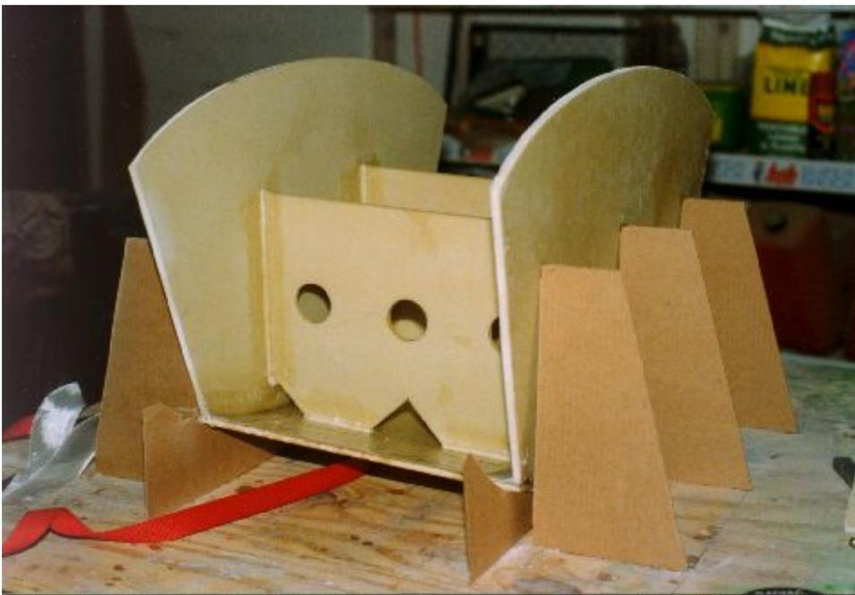
Here the baffles are installed. All seams are sealed with two plies of 2" wide fiberglass tape with flox (ground cotton in resin) used to radius all corners.
