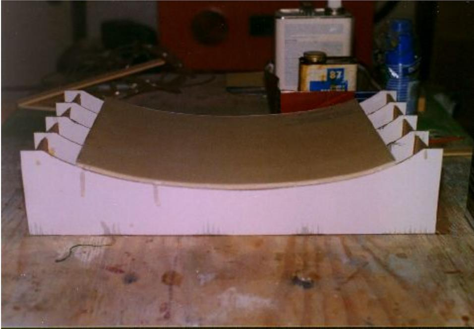
This is the bottom of the tank with two layers of the #7781 cloth and vinyl ester resin applied and cured. Note cardboard form which set the curve in the panel when I was laying it up and now doubles as a jig to hold the panel while I assemble the tank.
