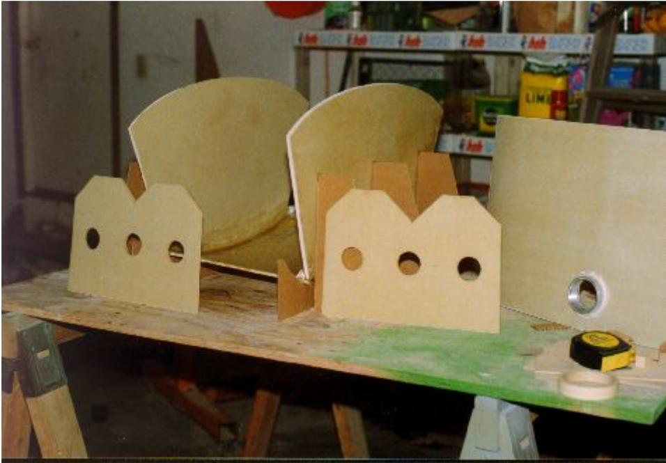
Here's a shot of the bottom panel now with the end panels in place. Also shown are the two baffle panels (the ones with the holes in them) and the top of the tank with aluminum fuel filler neck visible in the right of the picture. The baffle panels are sitting upside down. Note the notches cut in these panels. This is to allow fuel to flow to the bottom fitting even when aircraft is banking or pitching.
