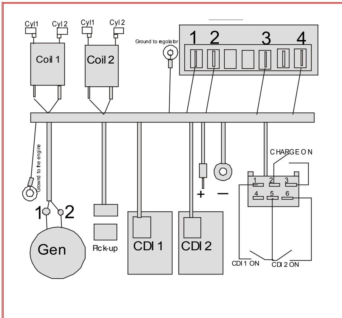
**The white connector must be connected as shown in the drawing:**
