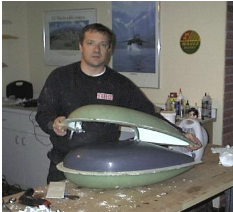
Here I am just as I released the 1st half of the mold from the plug.
