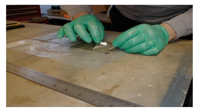
Once the cloth is in place use your razor blade to remove the remaining layer of plastic from the fiberglass cloth.
