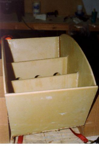
Tapes are wetted out and peel plied. I should mention here the importance of peel ply. It is used on all panel surfaces and tapes to insure the fibers are properly wetted out and laying flat which prevents fuel from wicking along the fibers and finding a path out of the tank.
