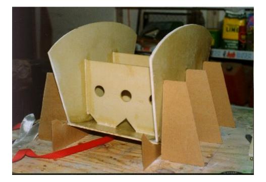
Here the baffles are installed. All seams are sealed with two plies of 2" wide fiberglass tape with flox (ground cotton in resin) used to radius all corners.
