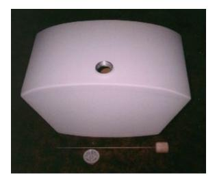
This is what all the work was for. Here's a shot of the completed tank from overhead. The fuel cap and float are at the bottom of the picture. The tank is sporting about \$20 worth of the new water based "Smooth Prime" from PolyFiber. I bought a quart from Wicks for \$25 to try. Smooth Prime is a WATER based primer designed specifically to help fill pinholes in composite
