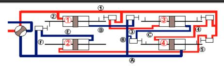
By proper connection of the sequencing valves and actuating cylinders, any sequence of events can be made to occur.
