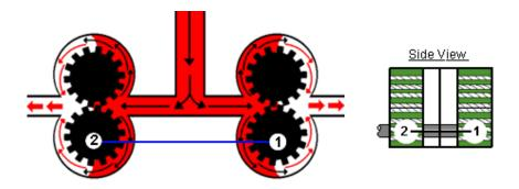
This kind of power pump is set between the two cylinders requiring equalization and would channel the flow to both cylinders (as shown below left). The VICKERS EQUALIZER setup is shown below right, where the VICKERS pumps are connected by a shaft at the center of the diagram. Input is at the top of the pumps and outputs are shown by the arrows.
