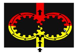
As the liquid comes from the reservoir, it is pushed between the gear teeth. The oil is moved around to the other side by the action of the drive gear itself and sent through the pressure line. What makes the oil squeeze in between the gear teeth? gravity and the pressure head. To prevent leakage of oil from the high to the low pressure side from occurring, you can make the gears fit better.
