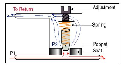
The adjustment screw at the top of the pressure relief valve is set for a certain pressure value, let us call it  $P_2$ . In general, even with a pressure of  $P_1$ , the poppet would lift up, except that the spring is strong and has downward force forcing the poppet closed. Poppet will not move until a pressure greater than that required is felt by the system (i.e.,  $P_1 > P_2$ ). When the pressure increases, the poppet will move up, forcing the excess
