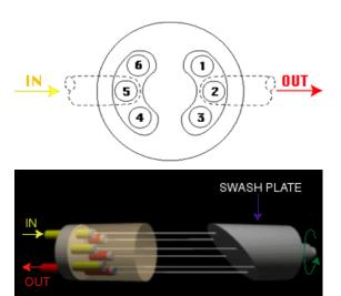
As the shaft and swash plate rotate, the piston will suck oil into the cylinder block and as the shaft and swash plate keep on rotating, the piston pushes oil out through the outlet. Pumps can be made to move more or less oil volume.
