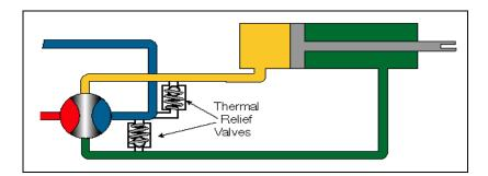
3. Force Limiting Device (FLD). Suppose that we want 1000 pounds of force to move a certain control surface. But our system can deliver 3000 pounds per square inch. If that pressure can be delivered on a 2 square inch piston head that moves the control surface, we would be= 6000 lb, a much higher force than is needed. We can put a force limiting relief valve (FLD) which would limit the force to 1000 lb by adjusting the FLD to act when the pressure reaches 500 psi
