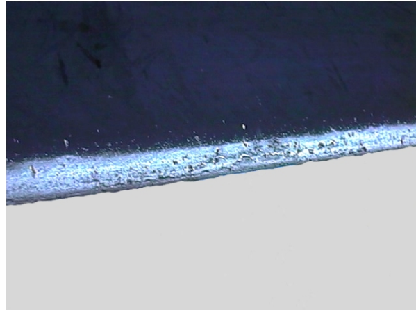
FIGURE 1-5. Exfoliation on the Blade Leading Edge
