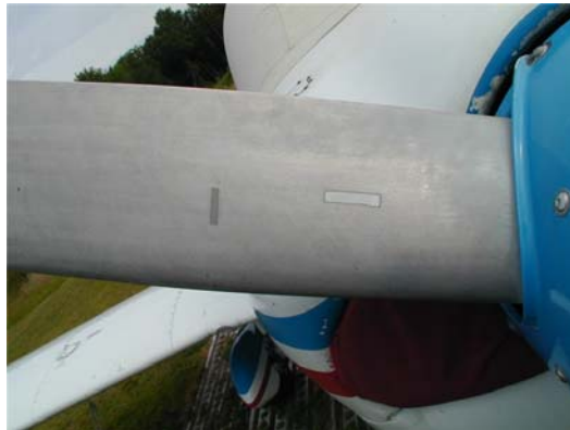
FIGURE 3-1. Balance Tape that was not Removed
