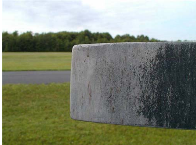
FIGURE 1-7. Erosion on a Metal Blade
