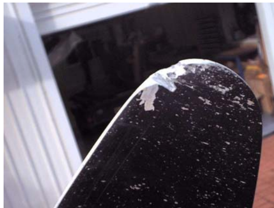
FIGURE 1-13. Propeller Blade Struck by a Foreign Object
