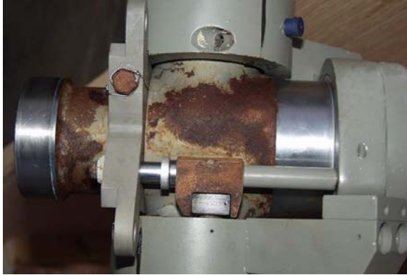
FIGURE 1-1. Hub Surface Corrosion
