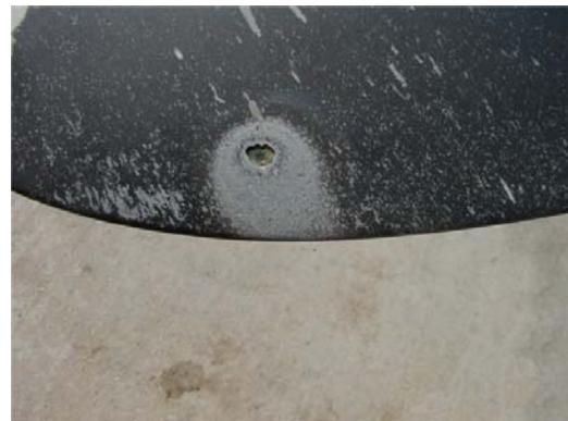
FIGURE 1-12. Lightning Strike on a Composite Surface
